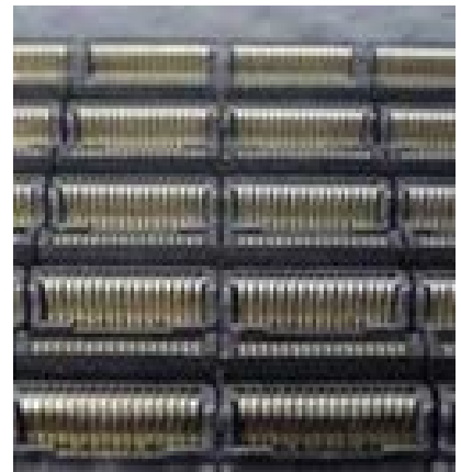
Test sockets are cleaned and restored with the RBP De-Ox process
