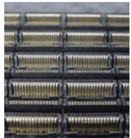
Test sockets are cleaned and restored with the RBP De-Ox process
